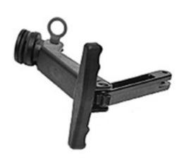
This over-centre T-handle style window hold-open is designed for top and side hinged venting windows and roof lights for on and off-highway vehicles. It is available with over-centre design (fully closed/fully open) or detented arm to position the window at intermediate positions and with or without a quick release pin.
